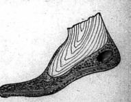
The new invention consists of the insertion of a mattress of canvas in which is embedded side by side a layer of narrow, flat, steel, springs. The canvas holds them in the pocket, in which they side freely, but the ends are capped with metal to prevent their perforating the rubber and leav-
