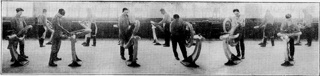
ment where National Speedway tires are built up by hand. In this department dozens of expert tire makers are em- from an actual photograph, shows the modern equipment of the splendid Pottstown plant.
