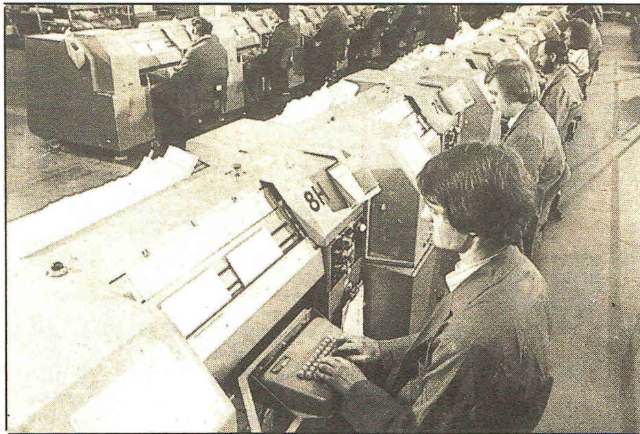
This new mechanical letter office means that operators can code up to 1,200 letters an hour.
